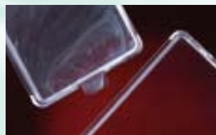
Blurry surface, caused by dust
