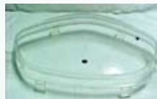
Black spots, caused by dust
