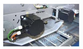
Curved cardboard blank ramp, slightly curved in its end sections allowing a smoother transfer of the flat blanks from the magazine to the packer's working plate.
