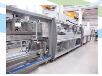
Externally-mounted energy-saving motors, which, thanks to the increased space created by the rounded sliding doors, are mounted on the machine's side edges allowing easy access for maintenance operations.
