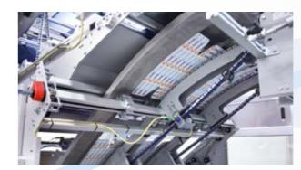
Automatic film-splicing system (optional), equipped with a high-performance welding bar which automatically joins and seals the edges of the two film reels with a 6-mm overlapping, making film positioning even easier and without using any double sided tape.
