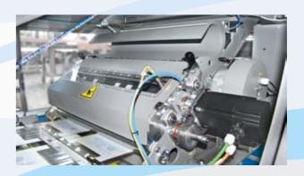
Film feed with built-in brushless motor, which enables a more precise and consistent film unwinding, especially during the film splicing operations. The absence of transmissions and switching devices means less parts to maintain.
