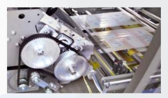
Direct drive film-cutting unit, equipped with direct drive motorization in order to improve the film-cutting precision and to reduce the frequency and complexity of maintenance interventions.
