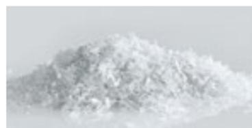
EU legislation on waste provides in future for higher collection amounts of PET bottles and mandatory high recycle content in PET bottles. VACUREMA® technology is ideal for the recycling of blow-moulded PET bottles from collection systems. Thanks to the patented pre-treatment of PET flakes, decontamination and IV increase is fast, reliable and thus effective and energy-saving.
