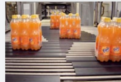
means of a translation device, with a maximum output of 80 packs per minute.
