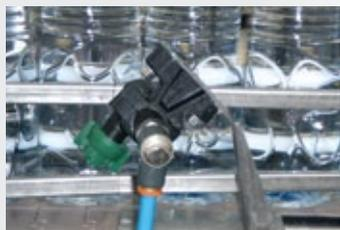
Smiline conveyors are lubricated by an automatic nozzle lubrication system, which minimizes the noise level, the operational costs and the cleaning interventions. It can be supplied “oil free” or
