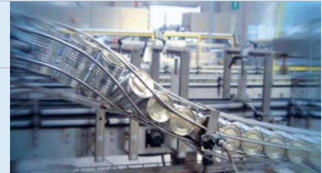
» **Additional cooling conveyor and pack turning device**
