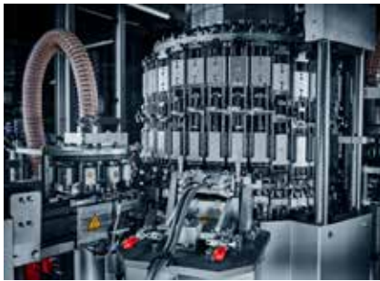
All functions integrated: assembly, slitting, folding, closing, checking, packing
