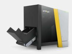
Preform monitoring during operation. The PreMon® inspects preform quality features in real time directly behind the injection molding machine. With the bad part ejector, the system actively improves the overall quality of an octabin or grid box. Due to its minimal footprint, the Pre-Mon® can easily be integrated between the injection molding machine and the packaging unit and with its active conveying concept, it guarantees a smooth production process.
