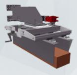
single column This two Cartesian axes, along which the horizontal beam slides up and down on ball recirculation guides.
