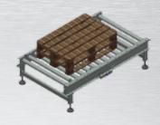
The APS palletizer is equipped with a system that feeds the empty pallets, and is made up of roller or chain conveyors (depending on the pallet's loading and releasing direction). Storage capacity: about 10 pallets for a total max height of 1700 mm.
