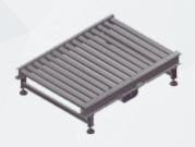
This is a galvanized steel structure with ø 76-mm rollers and 150mm pitch, motor driven by a 5/8" chain.
