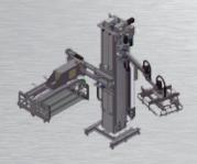
The "3-in-1" fixed column houses the mechanical parts designed to carry out the palletizing operations, feed the empty pallets and insert the interlayer pads, i.e. three processes usually carried out by separate
