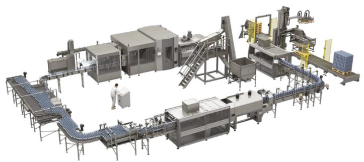
SMI offers complete bottling and packaging lines for production needs up to 33,600 bottles/hour intended for the food & beverages sector; designed in compliance with Industry 4.0 and IoT (Internet of Things) innovative principles, SMI plants can be considered as real "smart factories" thanks to the technological solutions of the latest generation they are equipped with.
