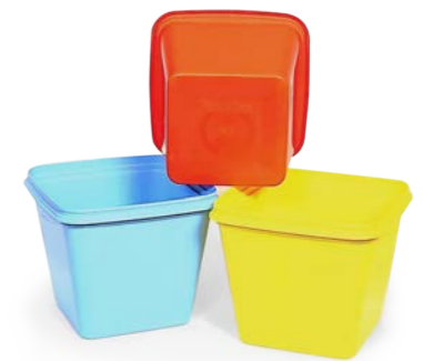
Rectangular containers produced by microcellular molding.
