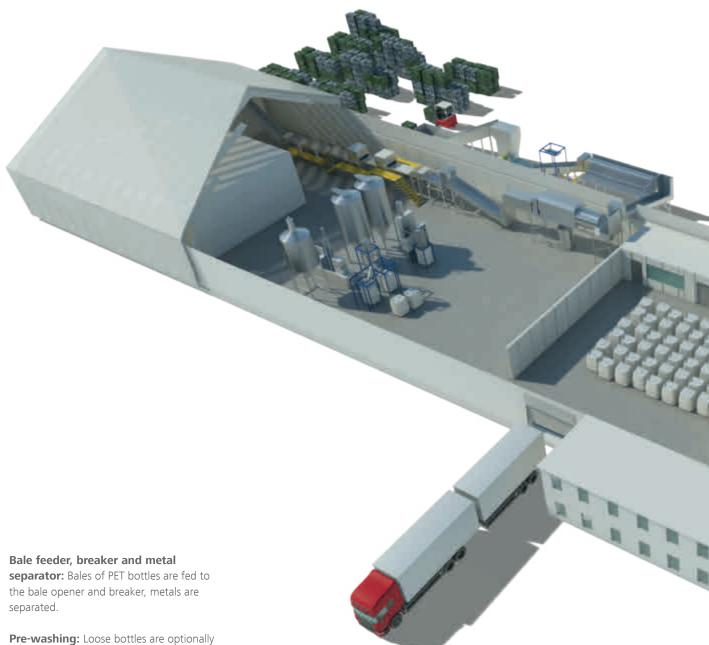
**Pre-washing:** Loose bottles are optionally pre-washed to improve the separation of PVC bottles and to remove labels.
