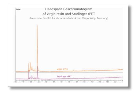
Frequent gas chromatography tests with rPET deliver better VOC results than virgin resin.
