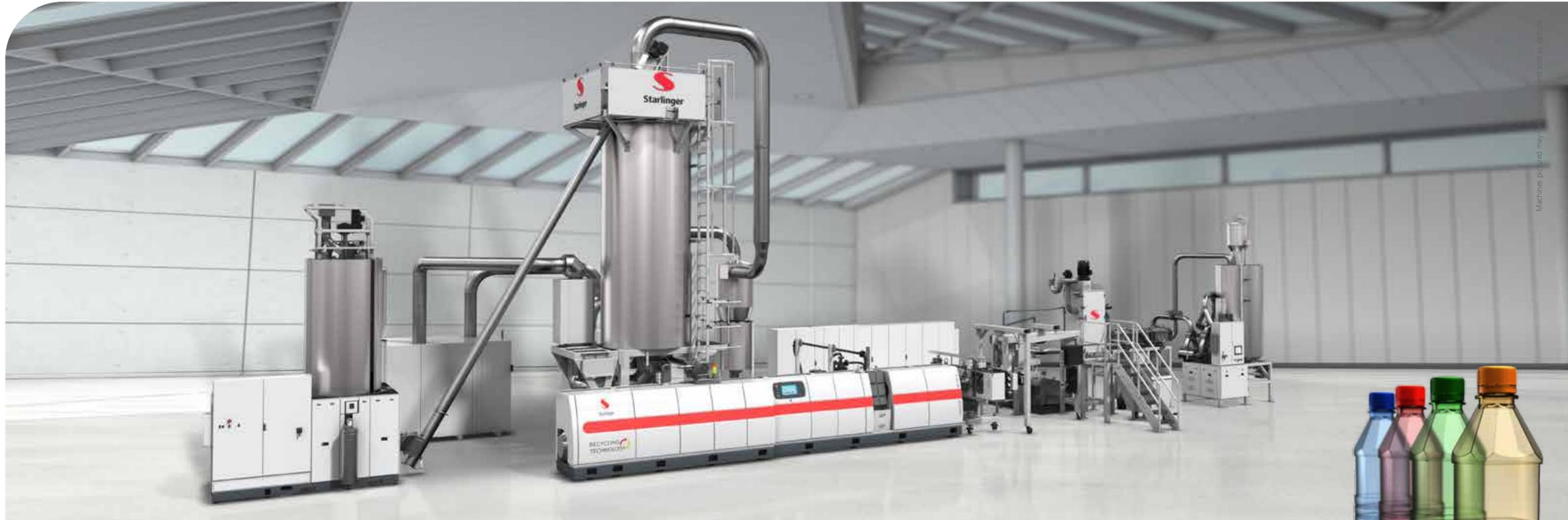
State-of-the-art recycling technology for the in-house recycling of PET flakes from bottles, preforms, strapping bands and sheets, as well as for the recycling of post-consumer bottle flakes after the washing process. The end product is melt-filtrated, uniform granulate that can be used for a wide range of food-contact applications.
