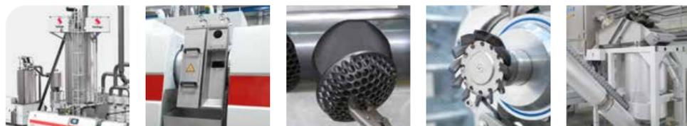
**The PET flakes** are fed into the pre-drying unit on top of the extruder. The material is dried, heated and crystallised, either by application of hot (desiccant) air, or vacuum. This treatment contributes a ready to outstanding decontamination results.
